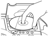
2 Press ▶|| on the unit (▶ on the remote) [8]. The unit plays all the tracks/MP3 files once. When you place MP3 discs, "MP3" appears in the display after the unit reads the file information.
