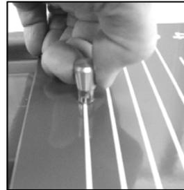
Pull Pin in Up Position (as seen from the bottom)
